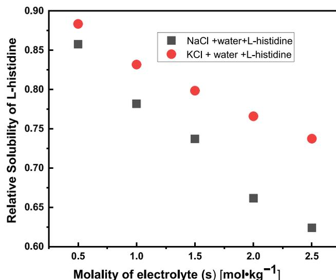
Fig. 4. Relative solubilities of L-histidine in NaCl + water (black) and KCl + water (red) solvent systems at 298.15 K. (For interpretation of the references to colour in this figure legend, the reader is referred to the web version of this article.)
