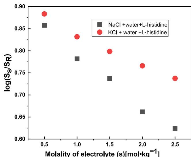
Fig. 5. Plot of logarithm of the ratio of solubilities  $S_s$  with and  $S_R$  without electrolytes for L-histidine in aqueous electrolyte (NaCl/KCl) mixtures in different composition at 298.15 K.
